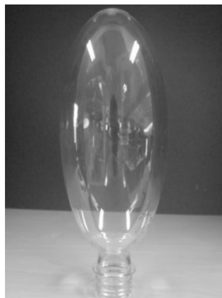
Figure 12 Final result of a free-blown preform after microwave heating.
